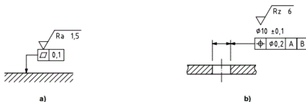
Figure 20 — Surface texture requirement — Geometrical tolerances indication
